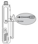
Attach/Remove the Antenna
